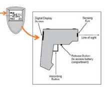
3. Give participants time to try measuring various surfaces with the infrared thermometer.
